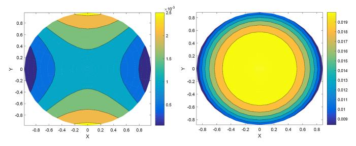
FIG. 3. Relative electric potential error from the pseudospectral method (left) and from the second-order finite difference method (right) inside a nearly round conducting pipe.
