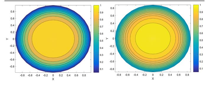
FIG. 2. Normalized electric potential distribution solution from the pseudospectral method (left) and from the second-order finite difference method (right) inside a nearly round conducting pipe.
